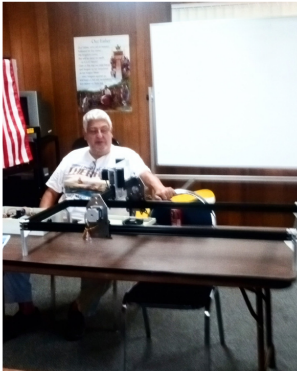
Scott brought in his laser cutter, this cutter can make 36" cuts in balsa wood, Nice toy Scott
