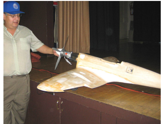
Scott Ramos brought in a Spitfire he is working on; it has an RCU .91 and a four blade prop for power.
